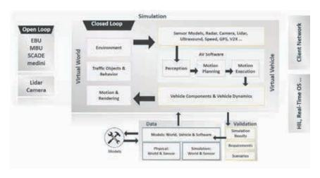
Figure 6. Illustration of the Ansys comprehensive solution for simulating autonomous vehicles miles driven.
